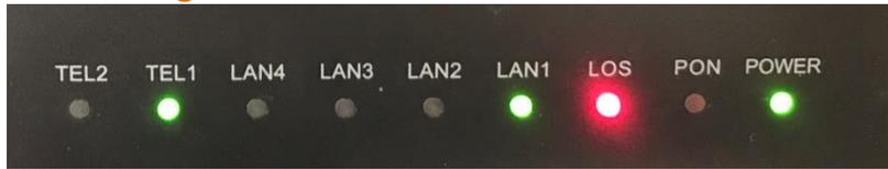
If the LED status for LOS shows red, please check whether the optical fibre is properly connected to the OPTICAL port and the Termination Port. If problem persists after a power cycle, please call our Customer Service at 1627.
